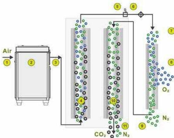
So far nothing new. Now the CO<sub>2</sub> is absorbed using desiccants in one of two Cartridges (4), with the desiccants in the cartridges having a defined life span.
